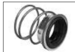
**3. MORE FLEXIBILITY WITH SEALS MEANS LONGER SERVICE LIFE.** Seals have more flexibility than packing and are able to compensate for shaft deflection, axial and radial end play, as well as vibration and wear of the sealing faces.
