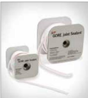
The original form-in-place gasketing, it's the most versatile and cost-effective alternative to sheet gasketing for large equipment flanges. Ideal for sealing complex surfaces, it conforms extremely well to rough or pitted surfaces. It's easy to install, too: just peel off the backing, apply to the surface, and overlap the ends for a remarkably tight seal.
