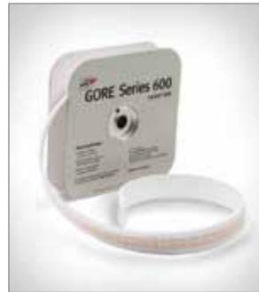
A form-in-place gasket for glass-lined equipment that guards against premature gasket failure. Unlike PTFE envelope gaskets, it won't degrade due to chemical attack, ensuring a tight, long-lasting seal. Made from 100% multi-directionally expanded PTFE, the entire gasket is chemically inert. It conforms to common glass-lined flange imperfections, yet maintains dimensional stability. Plus, installation is quick, easy and at lower cost.
